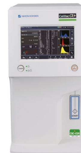
31 параметр: WBC, LY%, MO%, GR%, LY#, MO#, GR#, RBC, HGB, HCT, MCV, MCH, MCHC, RDW-CV, RDW-SD, PLT, PCT, MPV, PDW, P-LCR, P-LCC, Mentzer Index, RDWI, NLR, ESR, ESR HCT Corr., ESR TEMP Corr., SA, AMP, AI, MIN, t1/2
